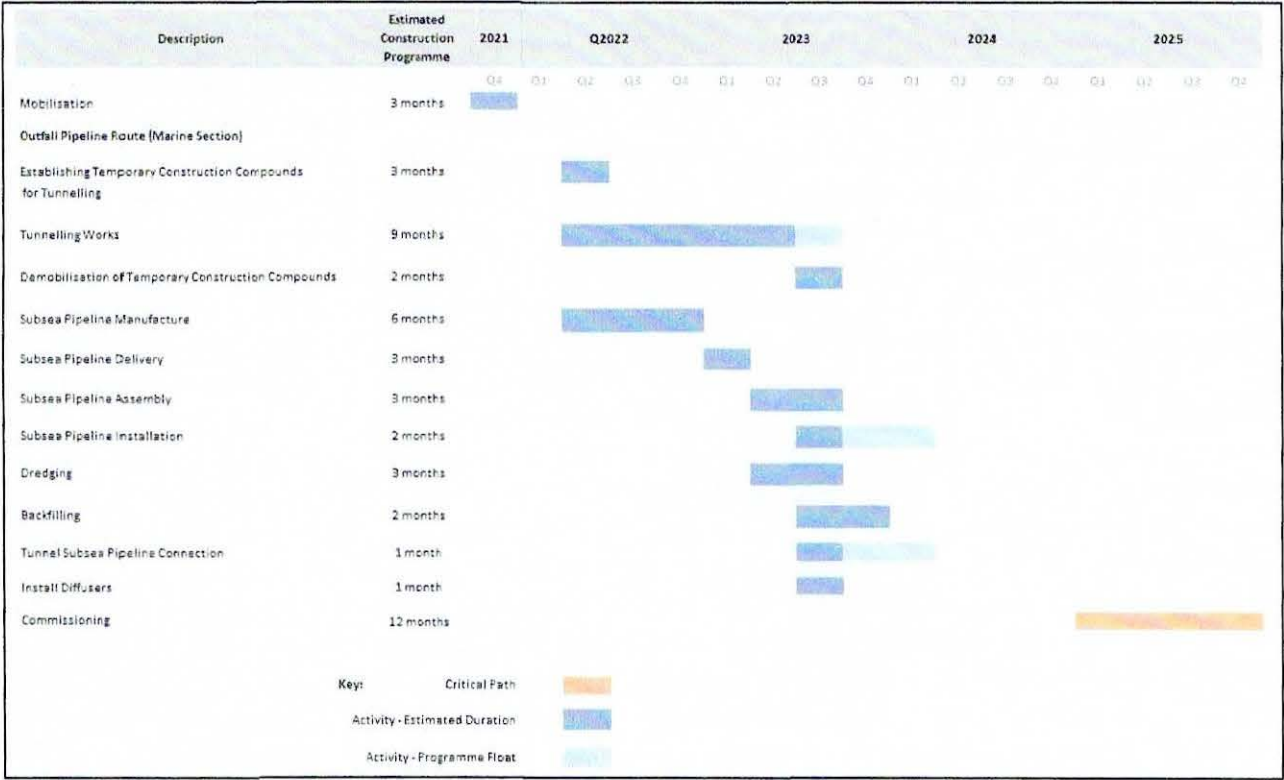
Figure 2: Outline Construction Programme–Marine Based Pipelines (Part of Overall Programme)
